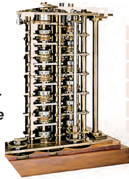
Difference Engine The completed portion of Charles Babbage's Difference Engine, 1832. This advanced calculator was intended to produce logarithm tables used in navigation.
